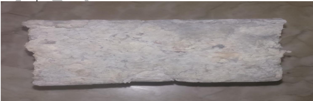
Figure 1: brick made up of waste paper pulp and cement.
